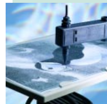
After checking that the drawing and cutting surface are correctly aligned, position the stylus at a convenient point on the drawing.
