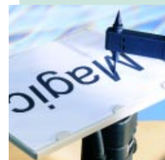
Signs, nameboards and logos can be reproduced, following a photocopy or computer print out. For these applications, use the parallel pin.
