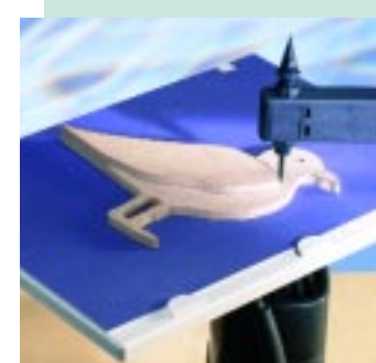
The parallel pin can also be used to follow two dimensional templates. Allow the pin to run lightly against the template edge to avoid any misalignment when changing direction.
