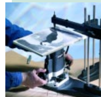
Start cutting by smoothly plunging the router to the cutting depth and following the line with the stylus.
